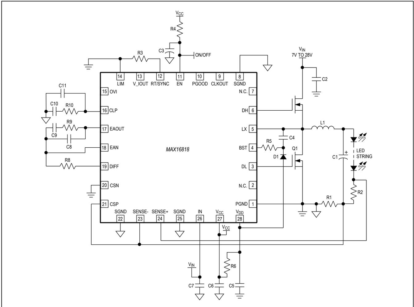
Figure 5. Application Circuit for a Buck LED Driver
