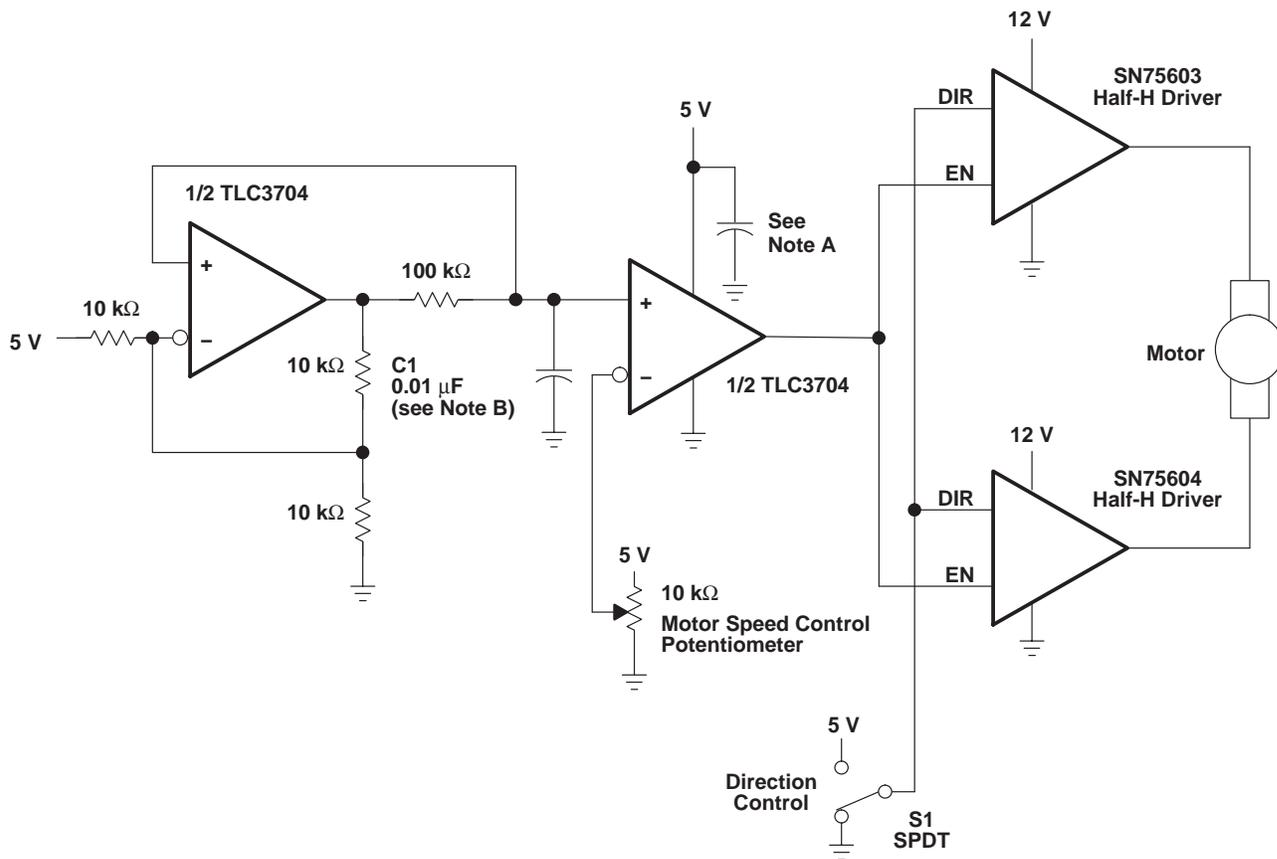
NOTES: A. The recommended minimum capacitance is 10  $\mu$ F to eliminate common ground switching noise.
