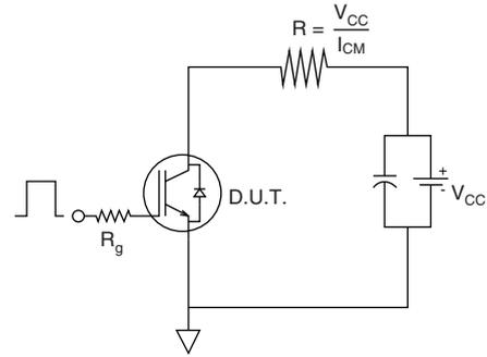
Fig. 18b - Pulsed Collector Current Test Circuit
