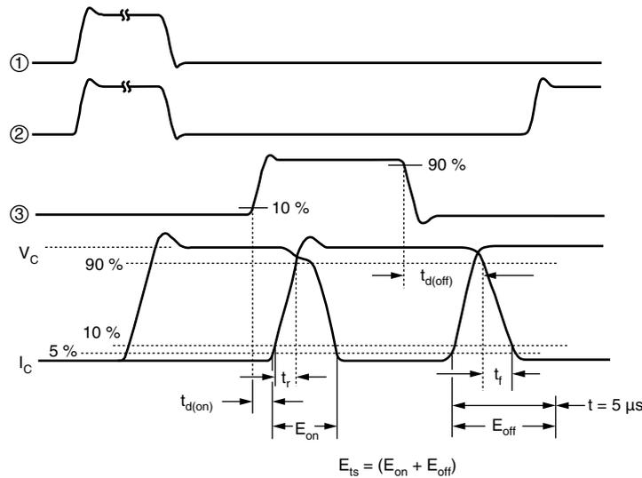
Fig. 19b - Switching Loss Waveforms Test Circuit
