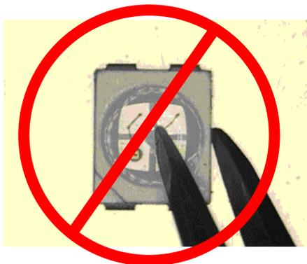
2) In general, LEDs should only be handled from the side. By the way, this also applies to LEDs without a silicone sealant, since the surface can also become scratched.
