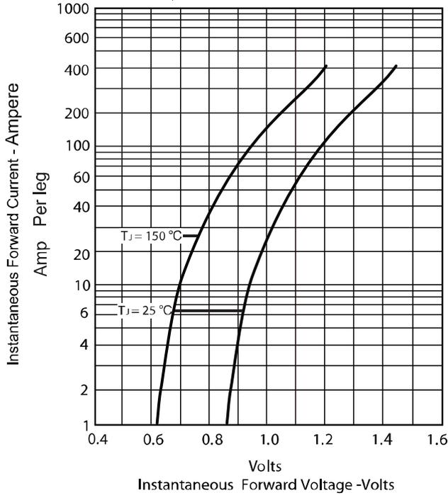
Figure.2 - Forward Derating Curve
