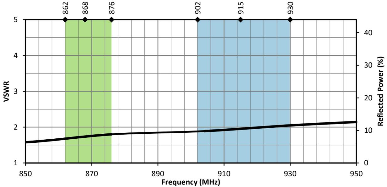
Figure 2. ANT- 8/9-VDP-2000 VSWR with Frequency Band Highlights
