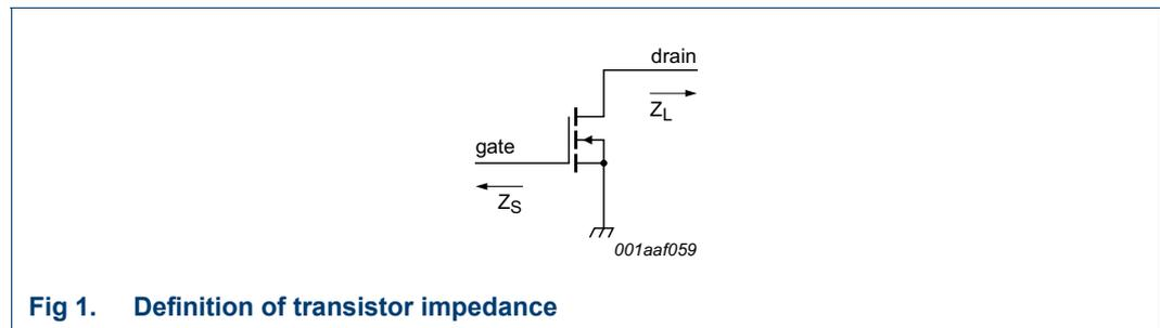
Fig 1. Definition of transistor impedance
