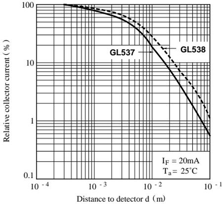
**Fig.10 Relative Collector Current vs. Distance (Detector : PD49PI)**
