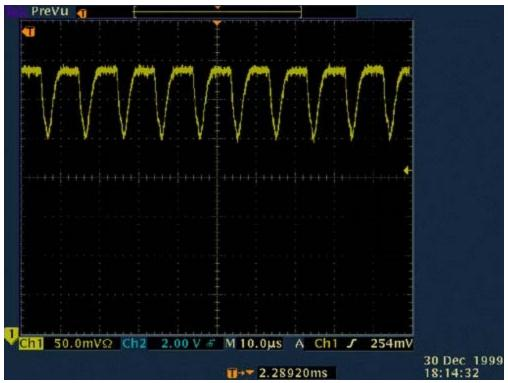
Figure 5. Decoupling capacitors tame the ringing in Figure 4.
