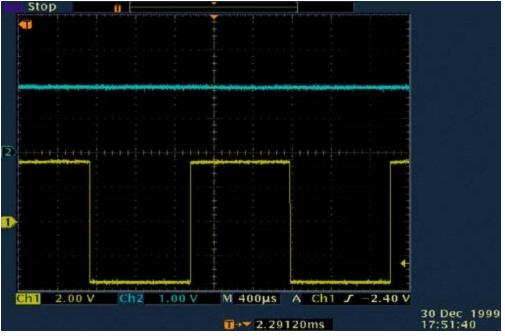
Figure 2. With a 2V input (top trace), this MAX3232 output (bottom trace) drives almost  $\pm$ 4V into an RS-232 receiver input.
