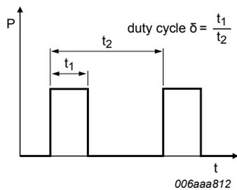
Fig. 18. Duty cycle definition
