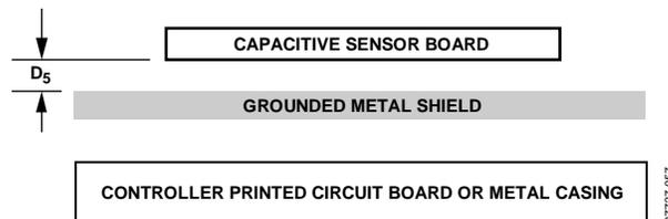
Figure 57. Capacitive Sensor Board with Grounded Shield
