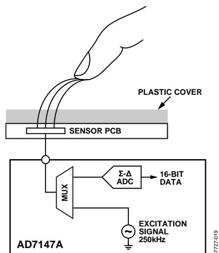
Figure 19. Capacitance-Sensing Method
