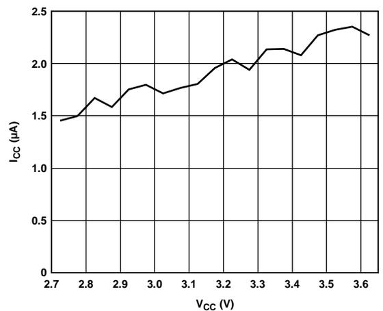
Figure 11. Shutdown Supply Current vs. Supply Voltage
