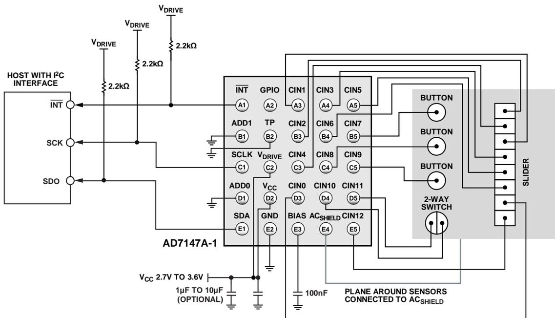
Figure 60. Typical Application Circuit with I2C Interface
