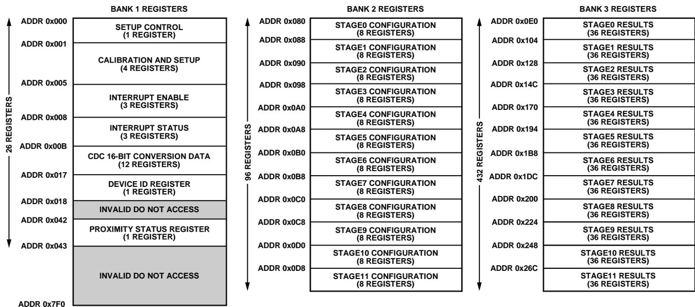
Figure 61. Layout of Bank 1, Bank 2, and Bank 3 Registers
