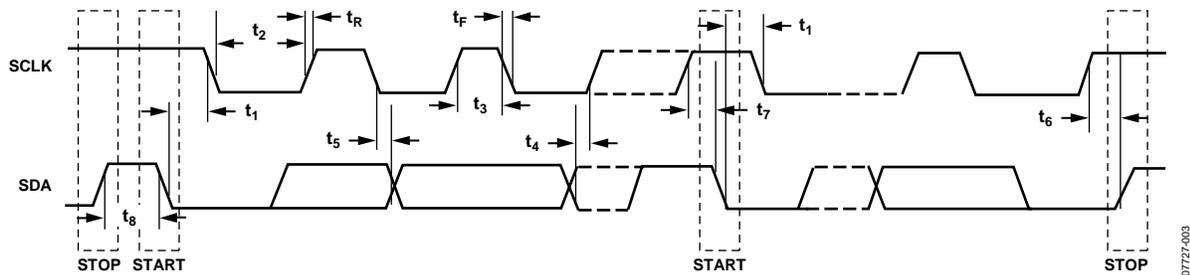
Figure 3. I<sup>2</sup>C Detailed Timing Diagram
