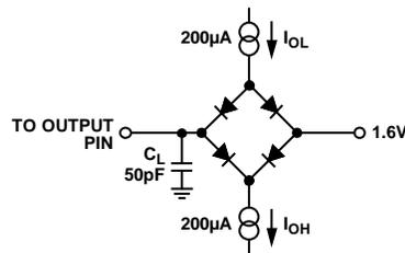
Figure 4. Load Circuit for Digital Output Timing Specifications
