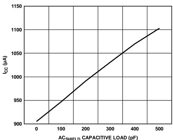
Figure 12. Supply Current vs. Capacitive Load on AC<sub>SHIELD</sub>
