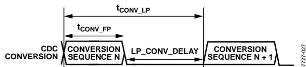
Figure 27. Low Power Mode CDC Conversion Sequence Time
