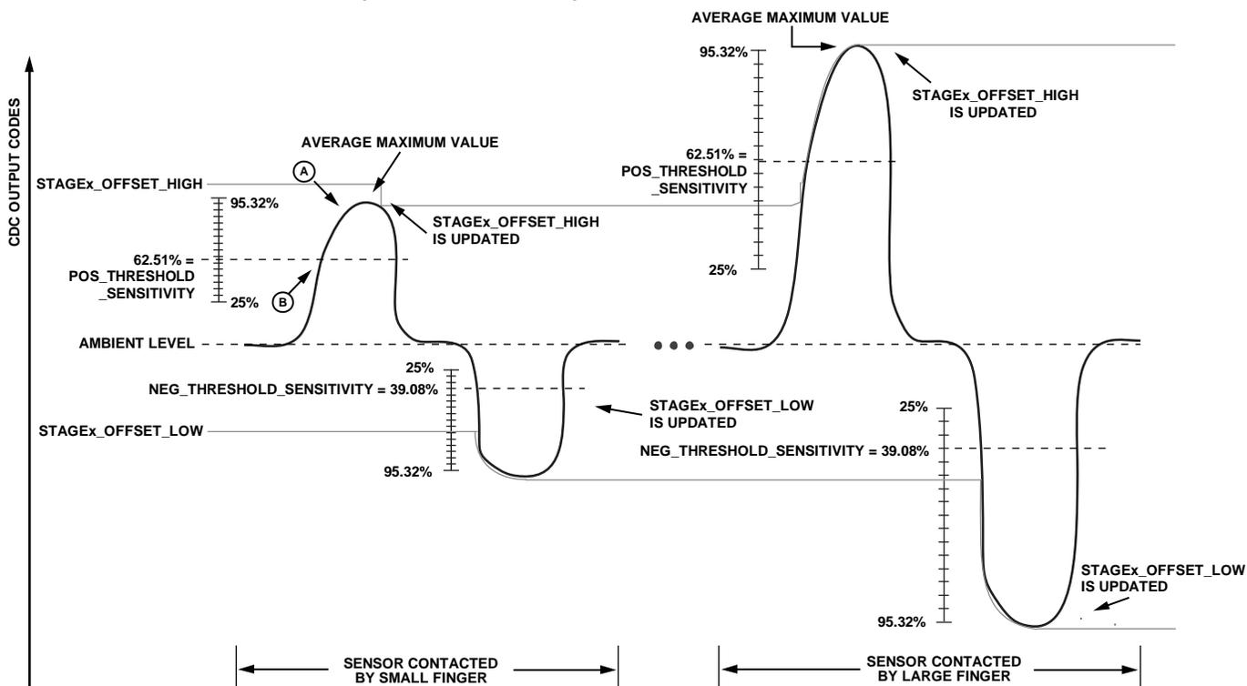
Figure 37. Example of Threshold Sensitivity (POS\_THRESHOLD\_SENSITIVITY = 1000, NEG\_THRESHOLD\_SENSITIVITY = 0011)
