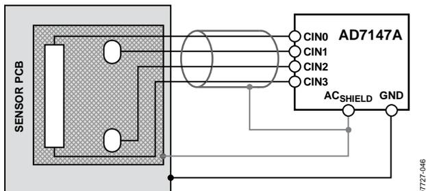
Figure 46. AC<sub>SHIELD</sub>
