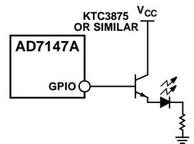
Figure 47. Controlling an LED Using the GPIO
