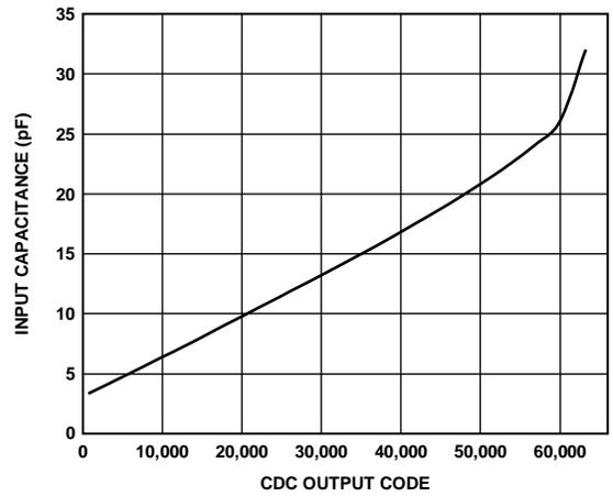
Figure 18. CDC Linearity,  $V_{CC} = 3.3 V$
