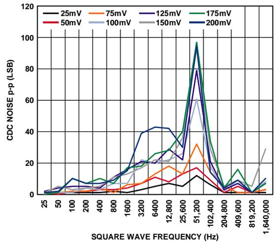
Figure 17. Power Supply Square Wave Rejection,  $V_{CC} = 3.6 V$
