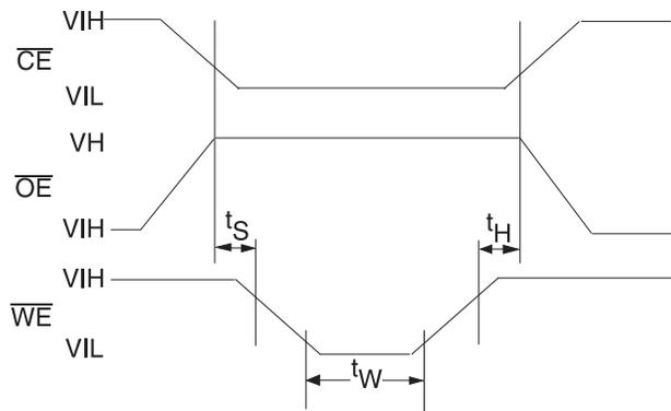
$t_S = t_H = 5 \mu\text{sec (min.)}$
