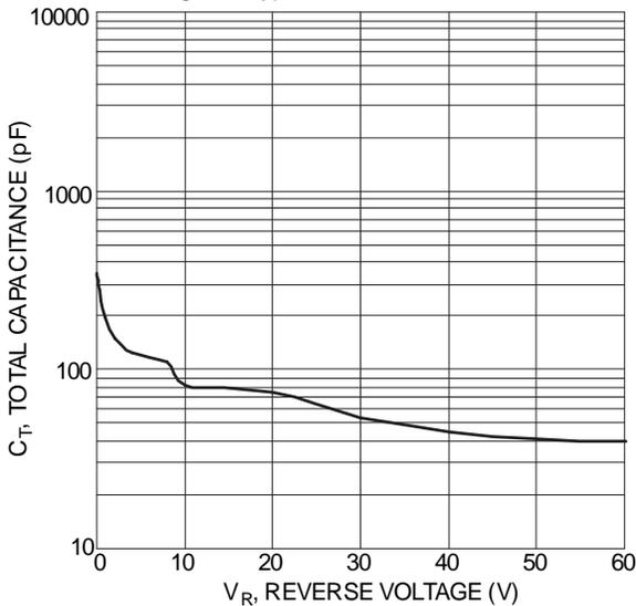
Figure 3 Total Junction Capacitance
