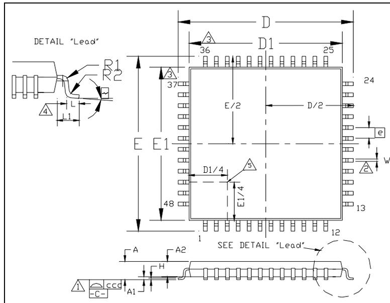
**Figure 8.17 - 48 Pin TQFP Package Outline**
