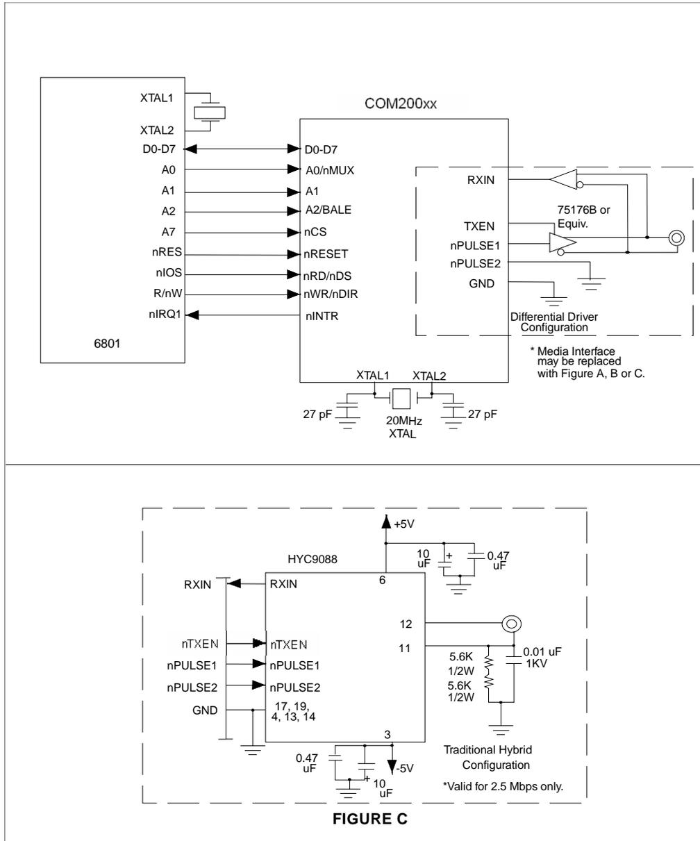
**Figure 5.2 - Non-Multiplexed, 6801-Like Bus Interface with RS-485 Interface**
