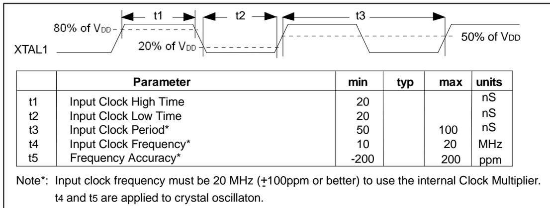
Figure 8.15 - TTL Input Timing on XTAL1 Pin
