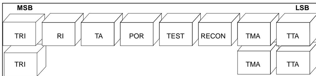
**Figure 6.3 - Command Chaining Status Register Queue**
