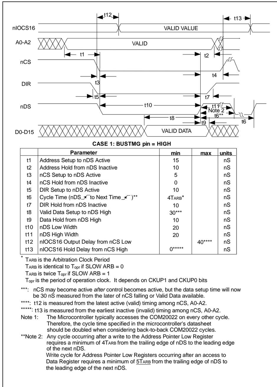
Figure 8.11 - Non-Multiplexed Bus, 68XX-Like Control Signals; Write Cycle
