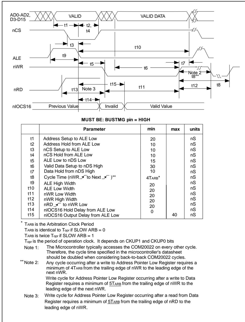
**Figure 8.4 - Multiplexed Bus, 80XX-Like Control Signals; Write Cycle**
