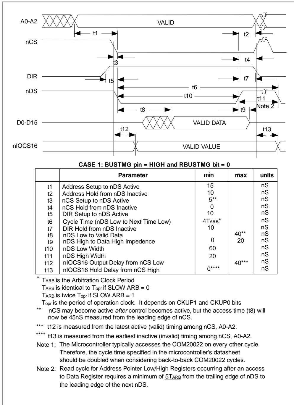
**Figure 8.7 - Non-Multiplexed Bus, 68XX-Like Control Signals; Read Cycle**
