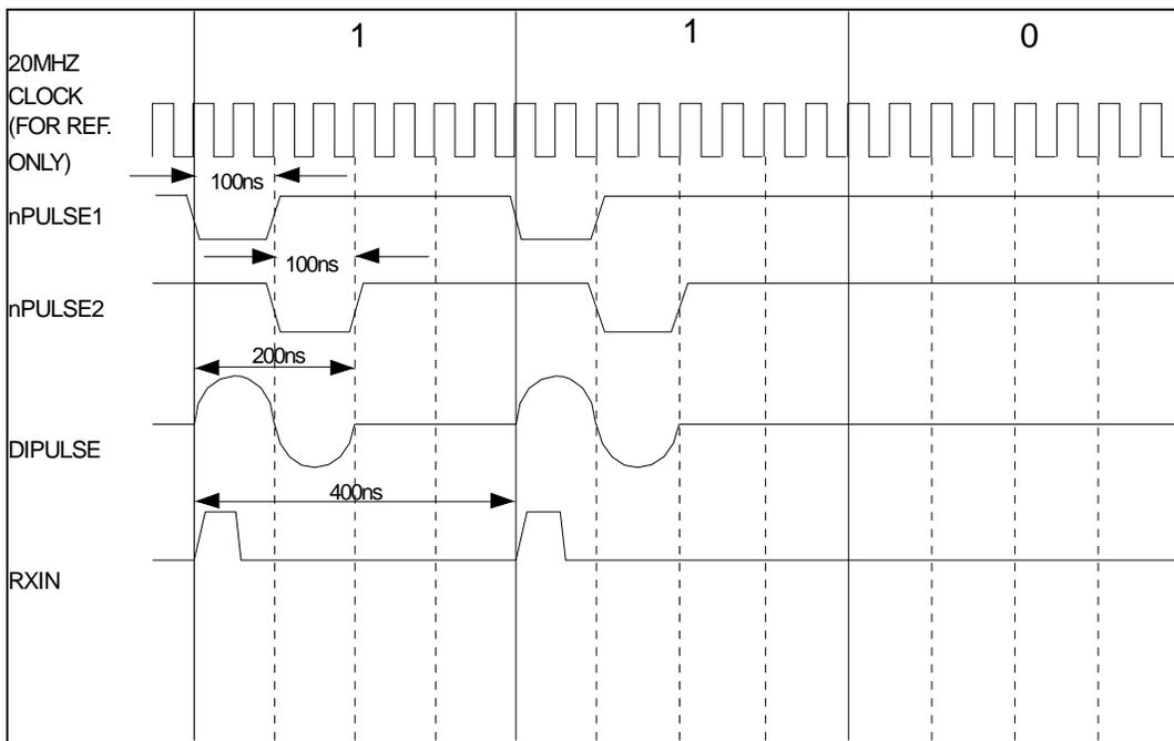
**Figure 5.5 - Dipulse Waveform for Data of 1-1-0**
