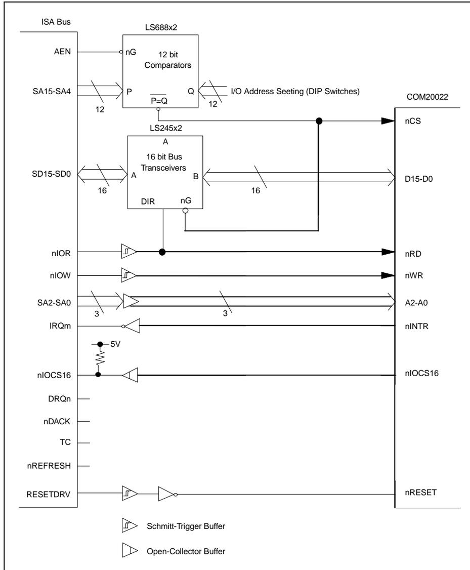
**Figure 10.1 - Example of Interface of Circuit Diagram to ISA Bus**
