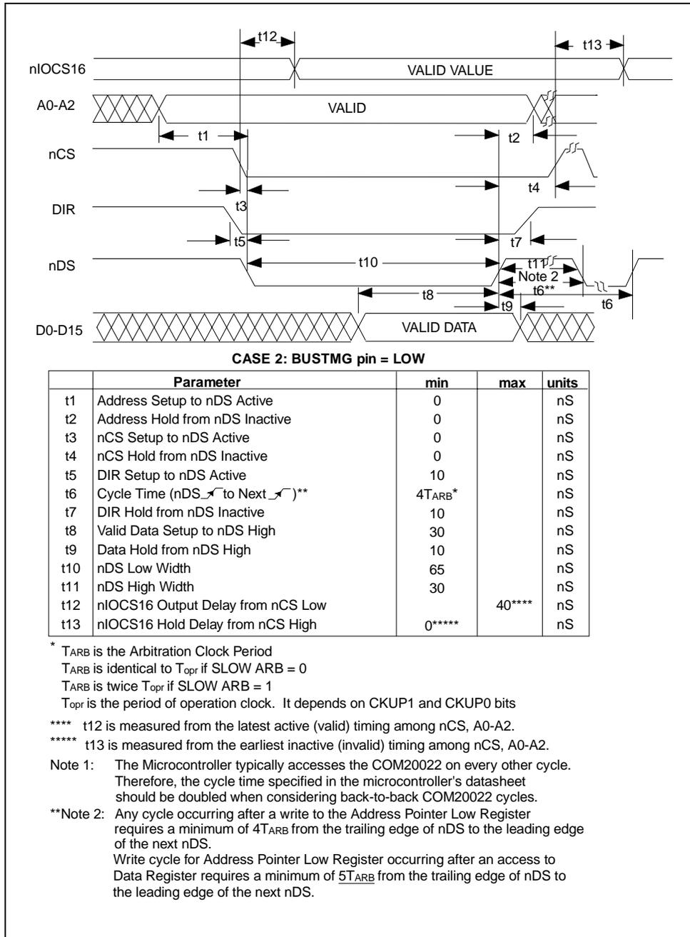
**Figure 8.12 - Non-Multiplexed Bus, 68XX-Like Control Signals; Write Cycle**
