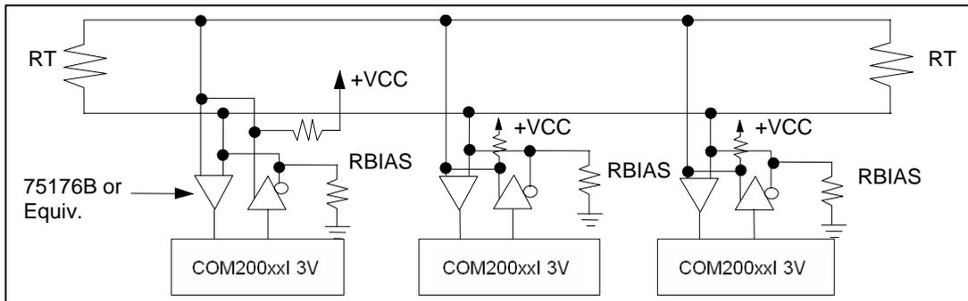
**Figure 5.4 - COM20022I 3V Network Using RS-485 Differential Transceivers**
