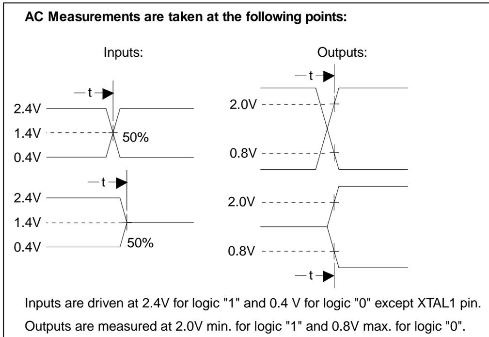
**Figure 7.1 - AC Measurements**
