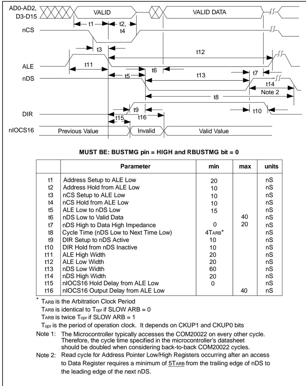
Figure 8.1 - Multiplexed Bus, 68XX-Like Control Signals; Read Cycle
