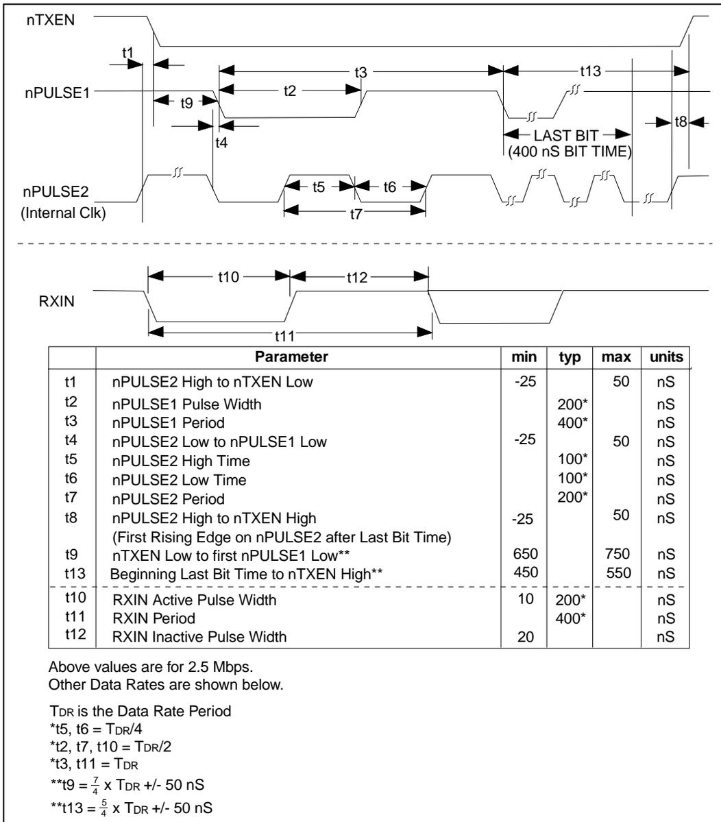
**Figure 8.14 - Backplane Mode Transmit or Receive Timing**
