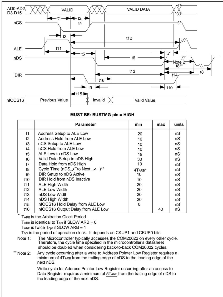
Figure 8.3 - Multiplexed Bus, 68XX-Like Control Signals; Write Cycle
