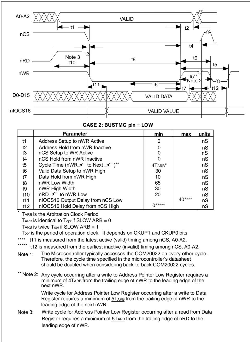
**Figure 8.10 - Non-Multiplexed Bus, 80XX-Like Control Signals; Write Cycle**
