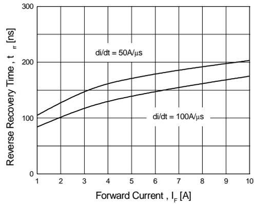
**Figure 4. Typical Reverse Recovery Time vs. Forward Current**
