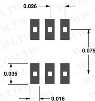
Figure 7. PCB Pad Layout (dimensions in inches).
