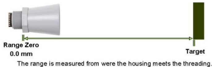
In general, the SCXL-MaxSonar-WRS self-cleaning sensors will report the range to the leading edge of the closest detectable object. Target detection has been characterized in the sensor beam patterns.
