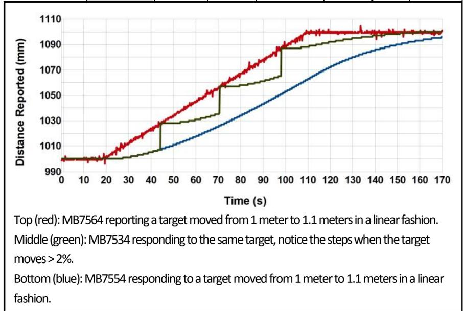
The MB7534 and MB7544 have an additional filter similar to the MB7554 and MB7574 except that the filter will reset to targets that are considered valid outside of a 2% distance to target window. This makes the sensor an ideal balance for accurately monitoring slow or stationary targets that occasionally move rapidly.
