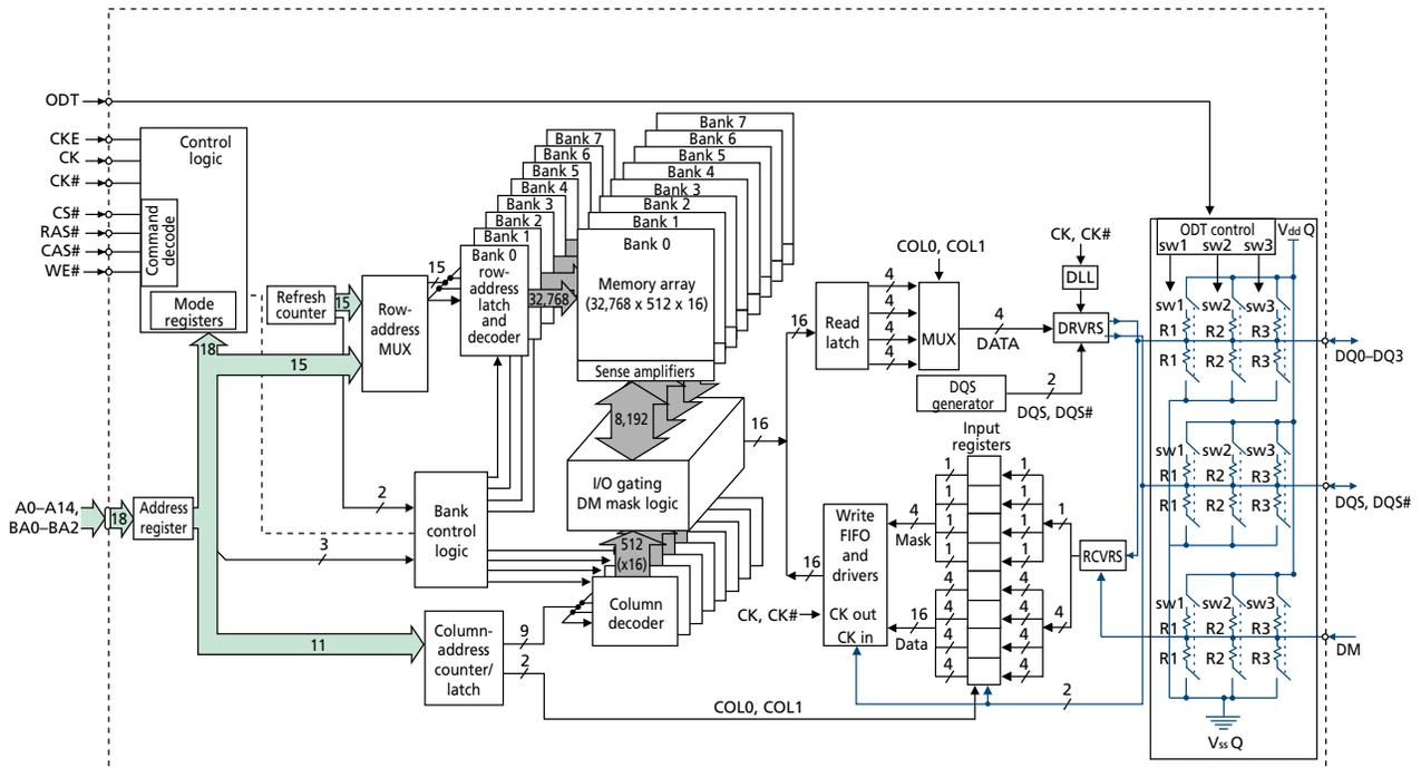
Figure 4: Functional Block Diagram – 256 Meg x 8
