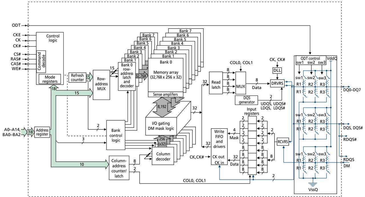
Figure 5: Functional Block Diagram – 128 Meg x 16
