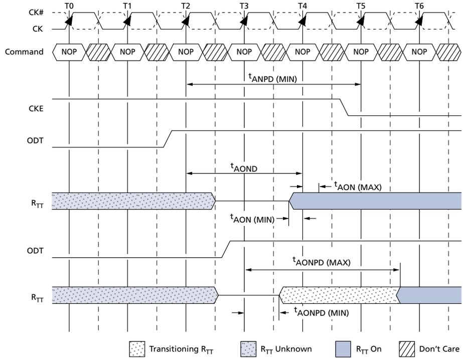
Figure 85: ODT Turn-Off Timing When Exiting Power-Down Mode
