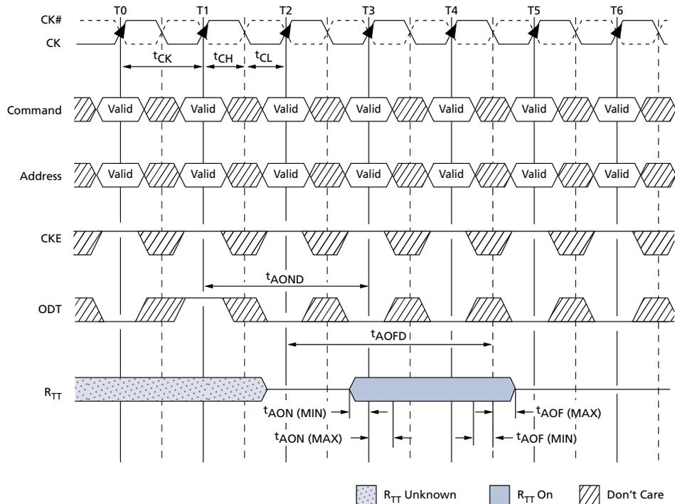
Figure 82: ODT Timing for Slow-Exit or Precharge Power-Down Modes
