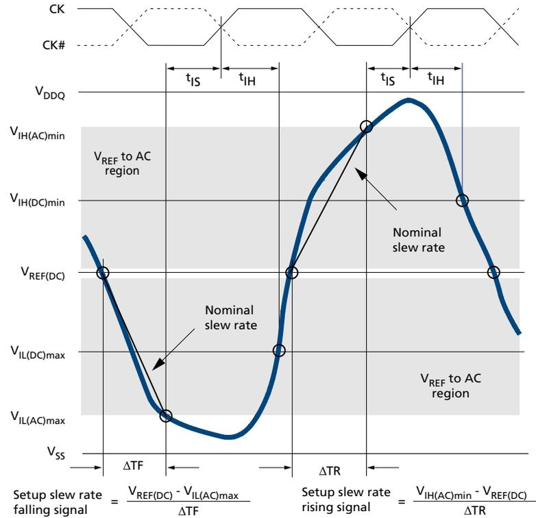
Figure 23: Tangent Line for  $t_{IS}$
