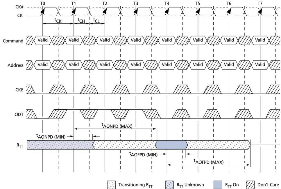
Figure 83: ODT Turn-Off Timings When Entering Power-Down Mode
