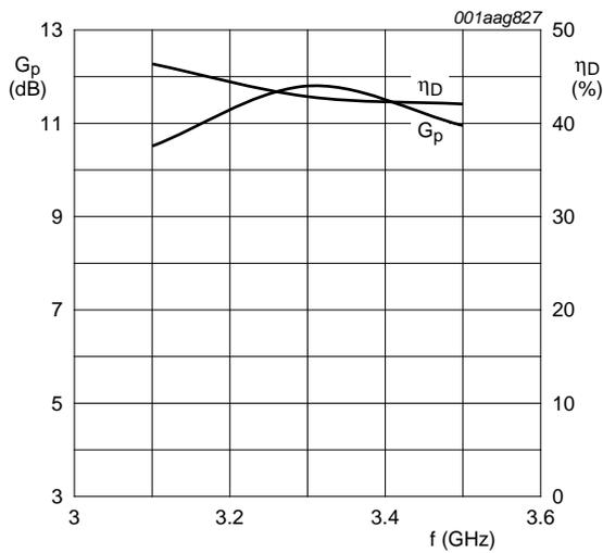
$V_{DS} = 32 \text{ V}; I_{Dq} = 100 \text{ mA}; t_p = 100 \mu\text{s}; \delta = 20 \%$ ;
