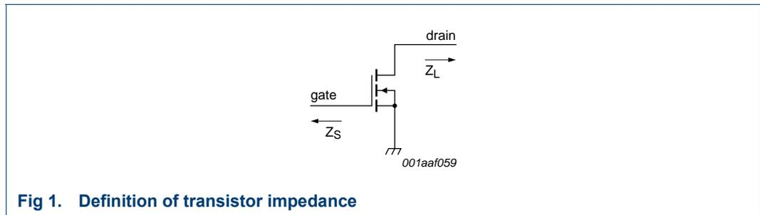
Fig 1. Definition of transistor impedance
