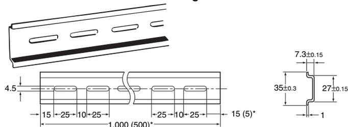
\* The dimensions given in parentheses are for the PFP-50N Socket Mounting Track.
