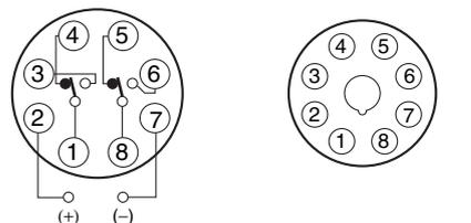
The polarity indication for terminals ② and ⑦ applies to the DC model (LG2-DB). (The above diagram shows the rear side of the Relay.)
