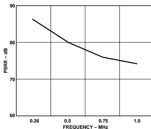
Figure 32. Power Supply Rejection Ratio of AD9754
