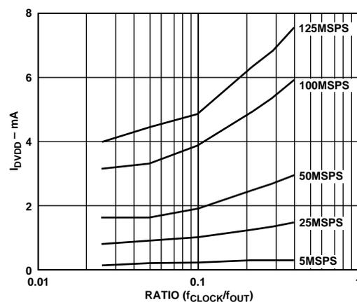
Figure 26.  $I_{DVDD}$  vs. Ratio @ DVDD = 3 V
