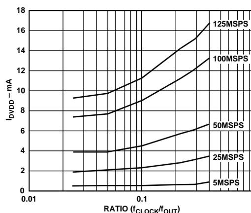
Figure 25.  $I_{DVDD}$  vs. Ratio @ DVDD = 5 V
