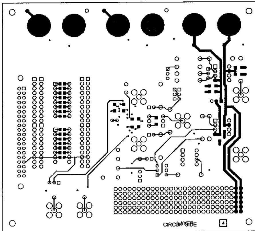
Figure 43. Solder Side PCB Layout (Layer 4)
