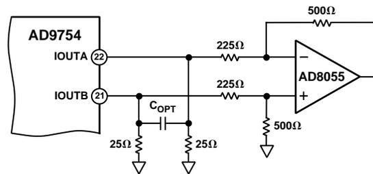
Figure 28. DC Differential Coupling Using an Op Amp
