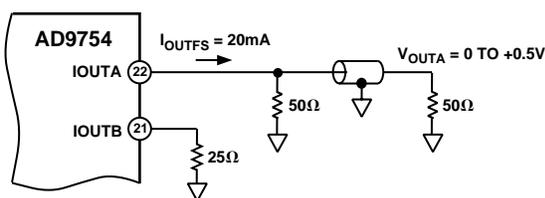
Figure 30. 0 V to +0.5 V Unbuffered Voltage Output
