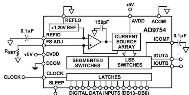
The AD9754 is a current-output DAC with a nominal full-scale output current of 20 mA and > 100 kΩ output impedance.
