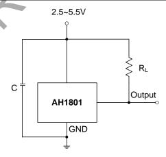
Notes: 4. C is for power stabilization and to strengthen the noise immunity, the recommended capacitance is 10nF to 100nF.  $R_L$  is the pull-up resistor, the recommended resistance is 10K $\Omega$  to 100K $\Omega$ .
