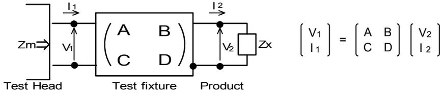
(2) The impedance of chip coil Zx and measured value Zm can be described by input/output current/voltage.
