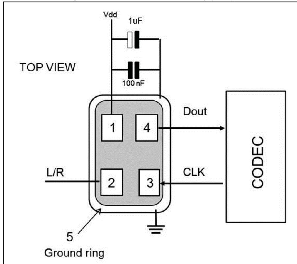
Figure 5: MP34DT05 electrical connections for stereo configuration (top view)
