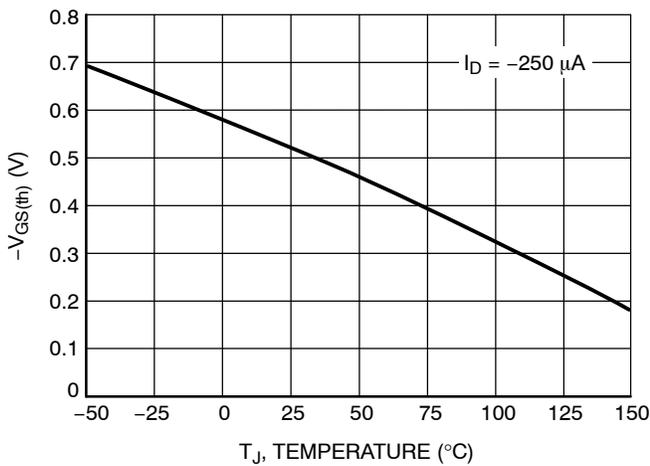
Figure 11. Threshold Voltage
