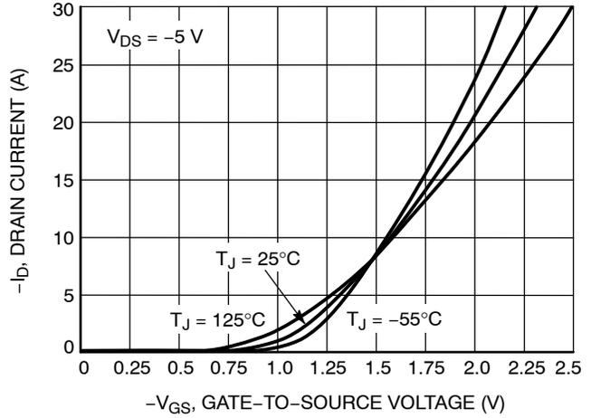
Figure 2. Transfer Characteristics
