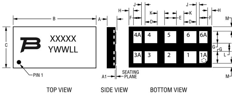
Pads 1A and 1 are internally connected; the same for pads 3A with 3, 4A with 4, and 6A with 6. This allows for one PCB layout to accommodate the Model P850.
