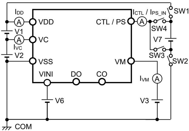
**Figure 7 Test Circuit 3**
