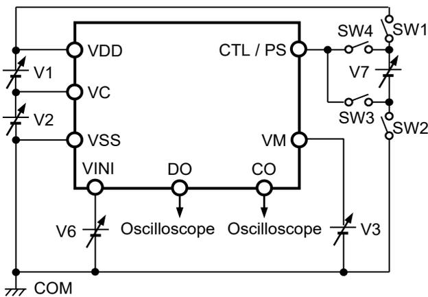
**Figure 9 Test Circuit 5**
