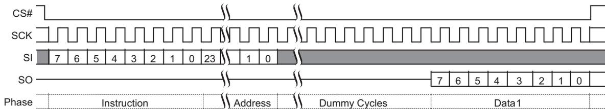
Figure 3.7 Dual Output Command
