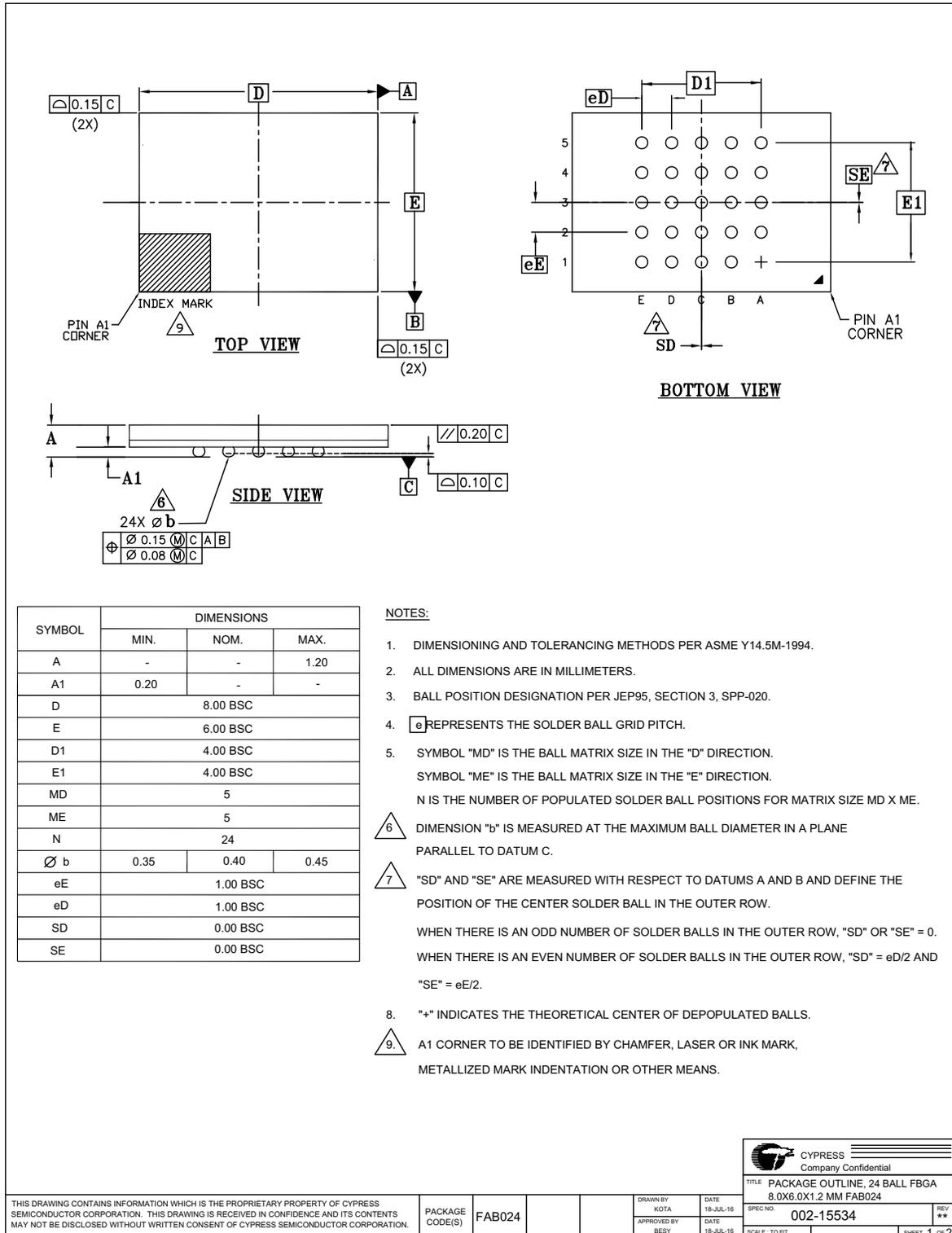
5.2.7 FAC024 — 24-Ball Ball Grid Array (8 mm × 6 mm) Package
