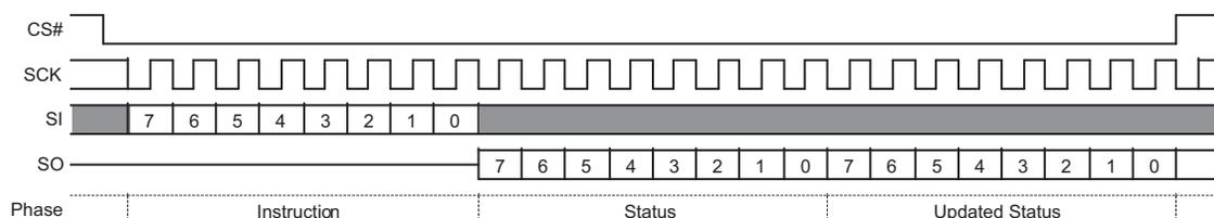
**Figure 8.2** Read Status Register-3 Command Sequence Diagram for 33h — S25FL132K / S25FL164K
