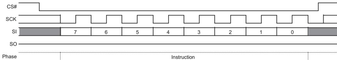
Figure 8.26 Read Electronic Signature (RES ABh) Command Sequence
