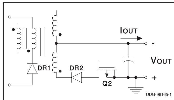
Figure 4d. Mode 4: Reverse power transfer, negative output.
