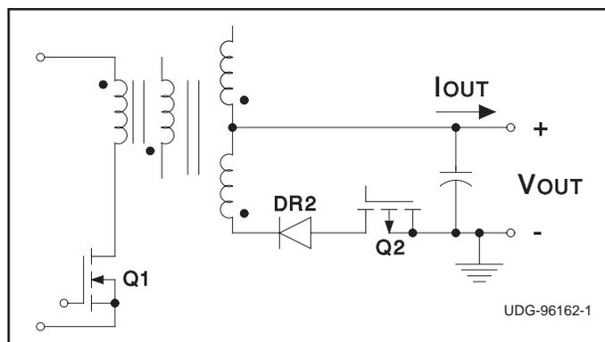
Figure 4a. Mode 1: Forward power transfer, positive output.
