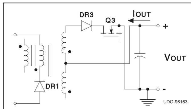
Figure 4b. Mode 2: Reverse power transfer, positive output.
