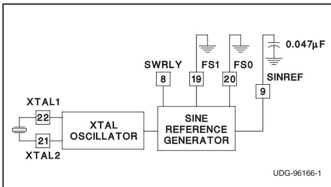
Figure 5. Sine-wave generator.
