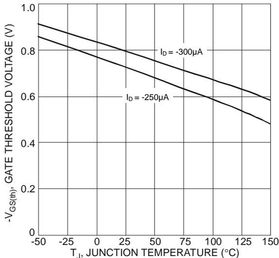
Fig. 19 Gate Threshold Voltage vs. Junction Temperature
