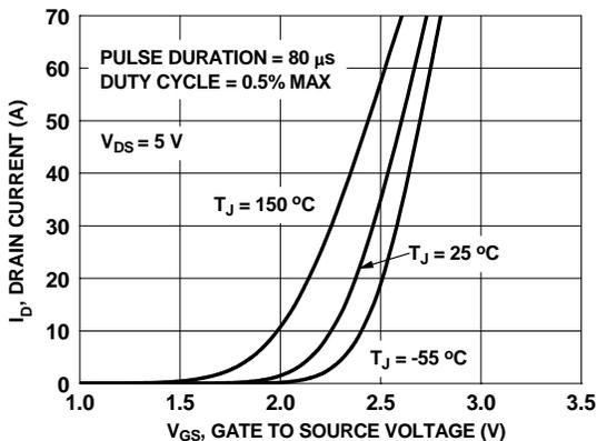
Figure 5. Transfer Characteristics
