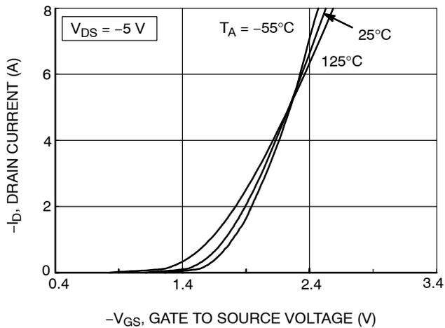
Figure 5. Transfer Characteristics
