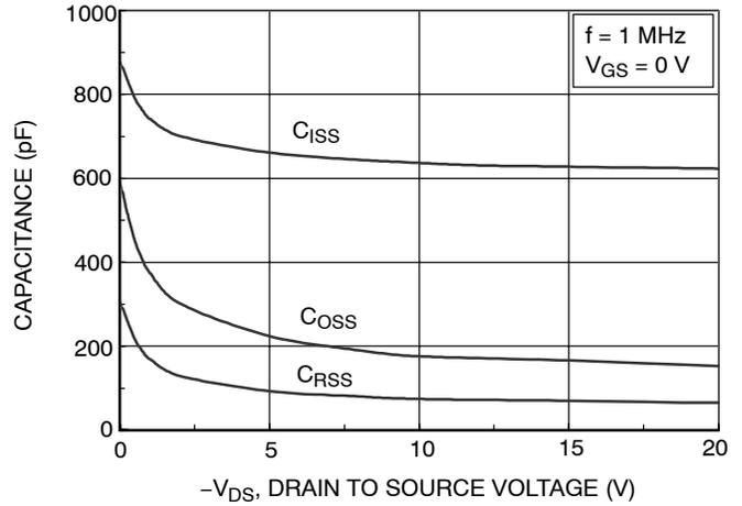
Figure 8. Capacitance Characteristics
