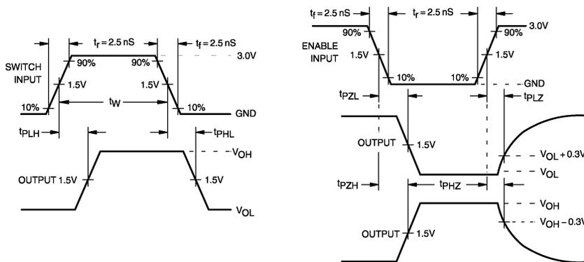
FIGURE 2. AC Waveforms
