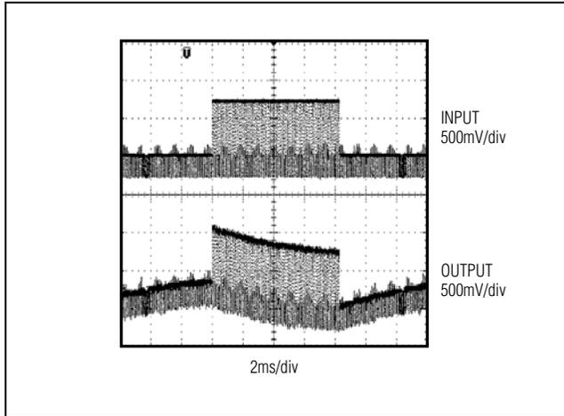
Figure 1. AC-Coupled Output
