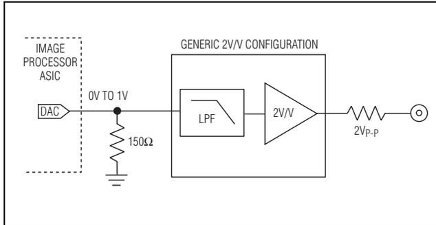
Figure 3. Typically, a Video DAC Generates a 1V<sub>p-p</sub> Signal Across a 150Ω Resistor Connected to Ground
