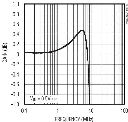
**NOTE:** GAIN VALUES (PLOTTED IN dB) ARE NORMALIZED VALUES RELATIVE TO THE EXPECTED VALUE OF 4V/V.
