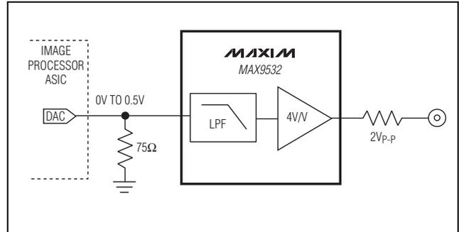
Figure 4. Video DAC Generates a 0.5V<sub>p-p</sub> Signal Across a 75Ω Resistor Connected to Ground
