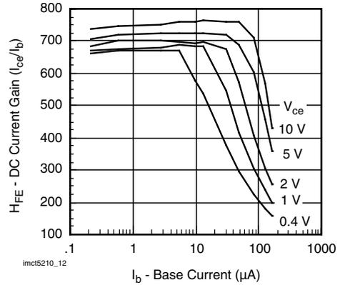
Fig. 12 - Transistor Current Gain vs. Base Current
