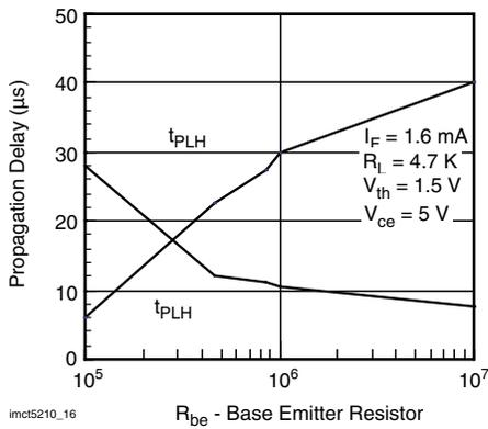
Fig. 16 - Propagation Delay vs. Base Emitter Resistor
