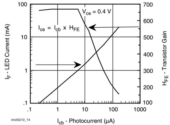
Fig. 14 - Transfer Curve
