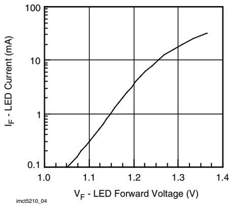
Fig. 4 - LED Forward Current vs. Forward Voltage
