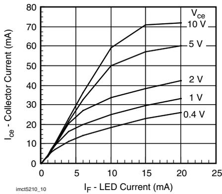
Fig. 10 - Collector Current vs. LED Current
