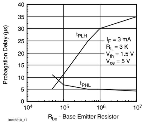
Fig. 17 - Propagation Delay vs. Base Emitter Resistor
