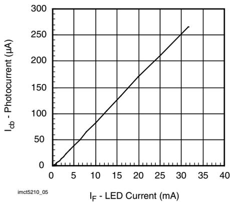
Fig. 5 - Collector Base Photocurrent vs. LED Current
