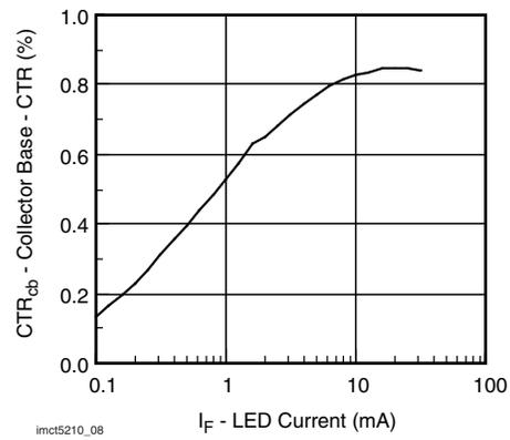
Fig. 8 - Collector Base CTR vs. LED Current
