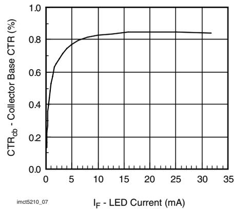
Fig. 7 - Collector Base CTR vs. LED Current
