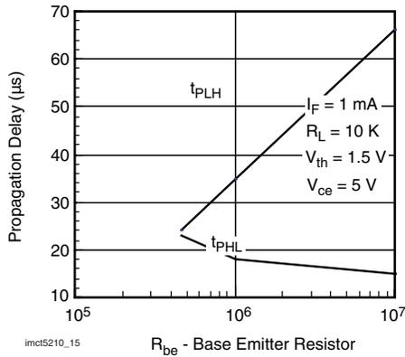
Fig. 15 - Propagation Delay vs. Base Emitter Resistor
