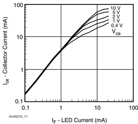
Fig. 11 - Collector Current vs. LED Current
