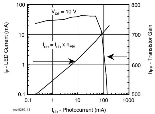
Fig. 13 - Transfer Curve
