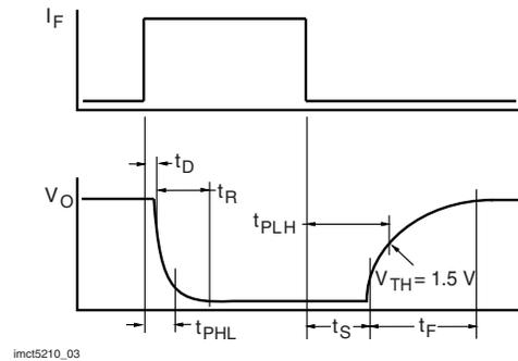
Fig. 2 - Switching Waveform
