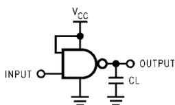
C<sub>L</sub> includes load and stray capacitance
