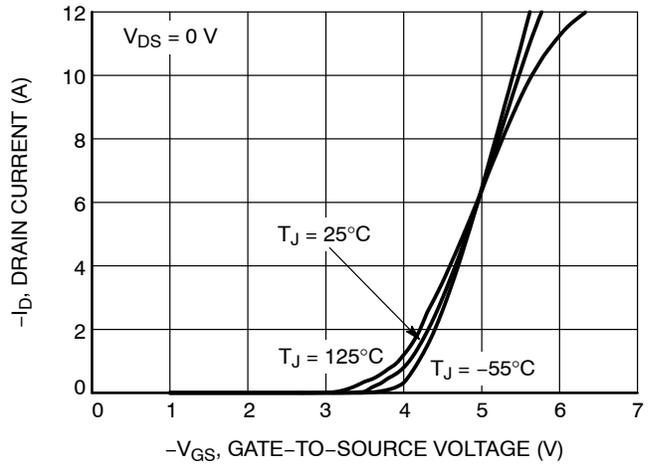
Figure 15. Transfer Characteristics
