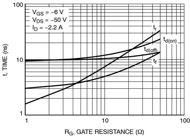
Figure 22. Resistive Switching Time Variation vs. Gate Resistance
