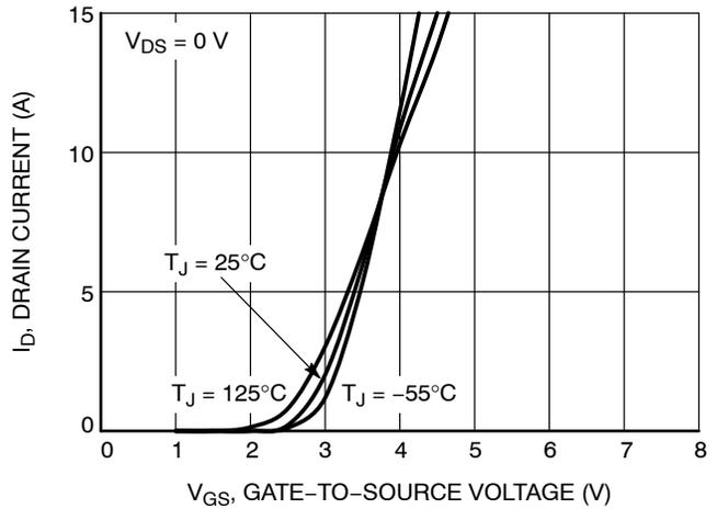
Figure 2. Transfer Characteristics
