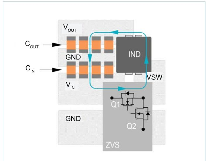
Figure 23 — Recommended component placement and metal routing
