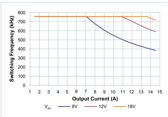
Figure 9 — Switching frequency vs. load current
