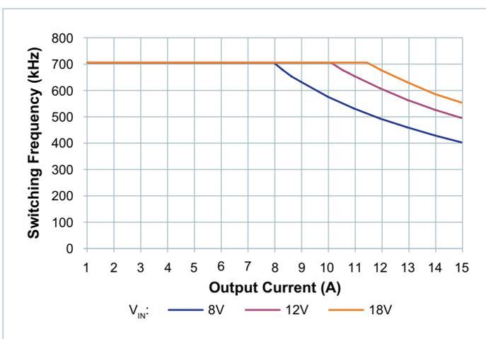
Figure 3 — Switching frequency vs. load current
