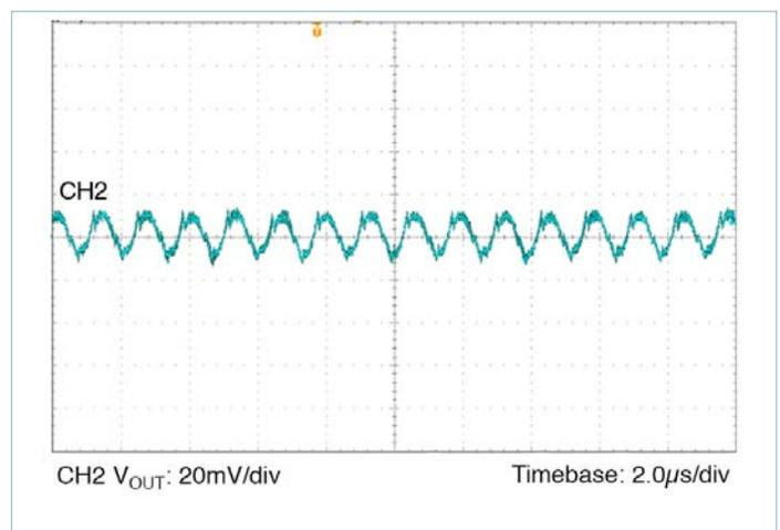
Figure 12 — Output ripple 12V<sub>IN</sub> 5.0V<sub>OUT</sub> at 7.0A; C<sub>OUT</sub> = 8 x 47μF
