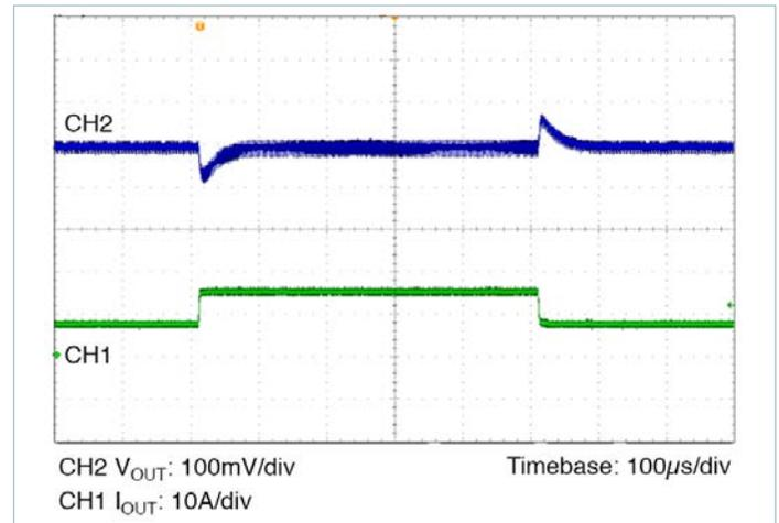
Figure 4 — Transient response: 7.5 – 15A, at 5A/μs
