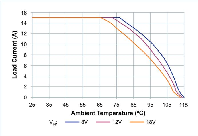
Figure 14 — PI3424 – load current vs. ambient temperature, OLFM
