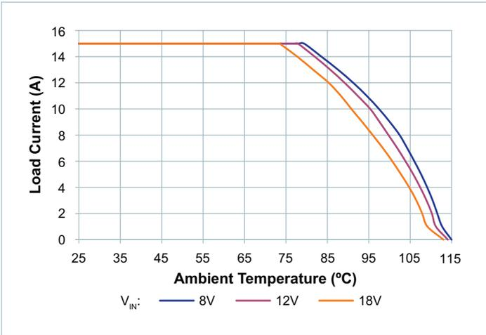
Figure 13 — PI3423 – load current vs. ambient temperature, OLFM
