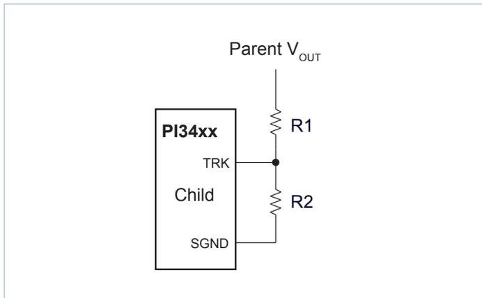
Figure 19 — Voltage divider connections for direct tracking
