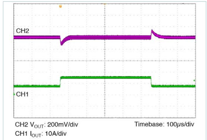
Figure 10 — Transient response: 7.5 – 15A, at 5A/μs
