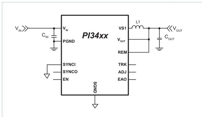
**Figure 15** — ZVS Buck with required components
