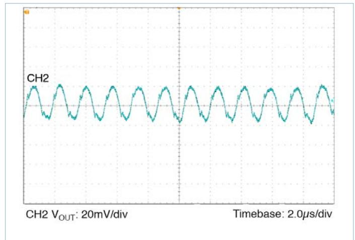
Figure 11 — Output ripple 12V<sub>IN</sub> 5.0V<sub>OUT</sub> at 15A; C<sub>OUT</sub> = 8 x 47μF
