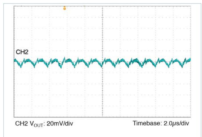
Figure 6 — Output ripple 12V<sub>IN</sub> 3.3V<sub>OUT</sub> at 7.0A; C<sub>OUT</sub> = 8 x 100μF
