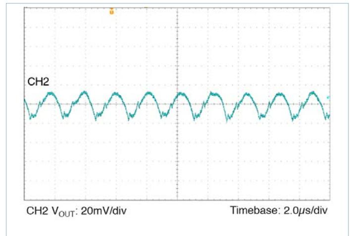
Figure 5 — Output ripple 12V<sub>IN</sub> 3.3V<sub>OUT</sub> at 15A; C<sub>OUT</sub> = 8 x 100μF
