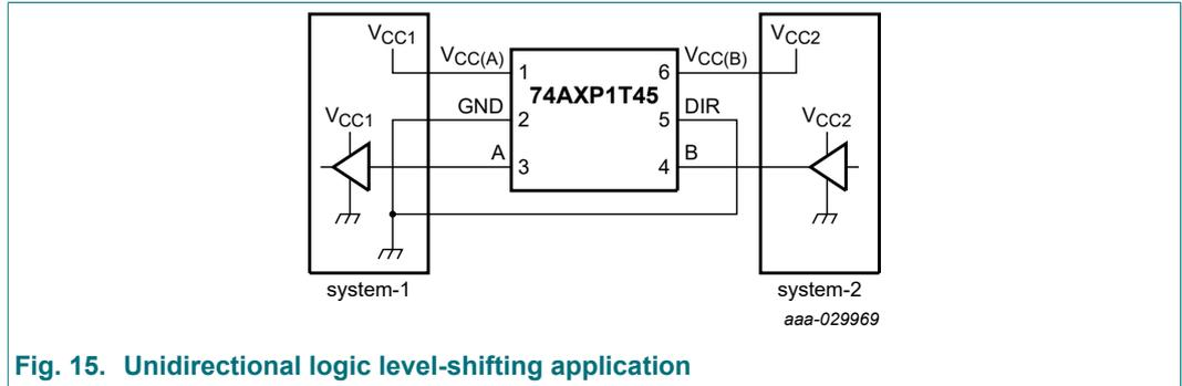
Fig. 15. Unidirectional logic level-shifting application
