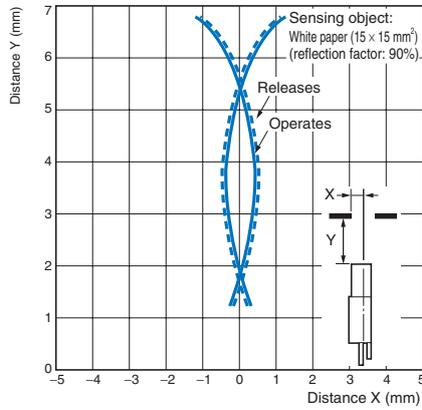
Sensing Distance vs. Object Area Characteristics
