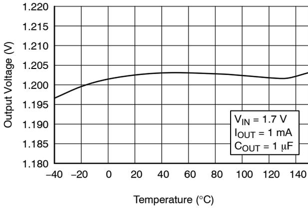
Figure 2. Output Voltage vs. Temperature –  $V_{OUT} = 1.2\text{ V}$
