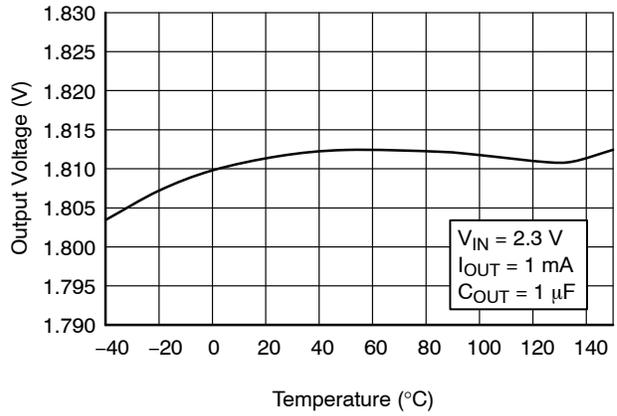
Figure 3. Output Voltage vs. Temperature –  $V_{OUT} = 1.8\text{ V}$
