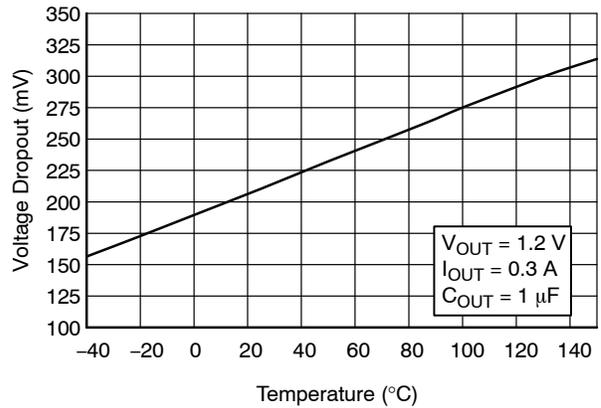
Figure 5. Dropout Voltage vs. Temperature –  $V_{OUT} = 1.2\text{ V}$
