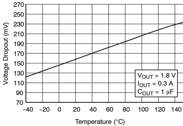
Figure 6. Dropout Voltage vs. Temperature –  $V_{OUT} = 1.8\text{ V}$
