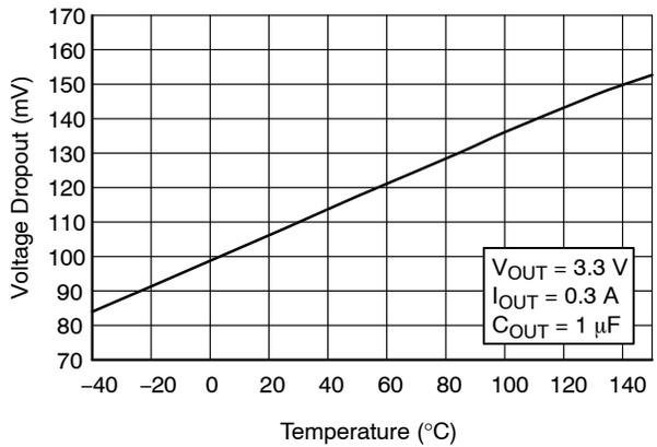
Figure 7. Dropout Voltage vs. Temperature –  $V_{OUT} = 3.3\text{ V}$
