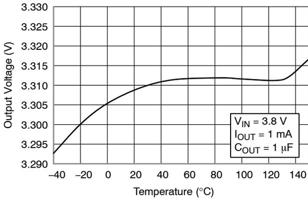
Figure 4. Output Voltage vs. Temperature –  $V_{OUT} = 3.3\text{ V}$
