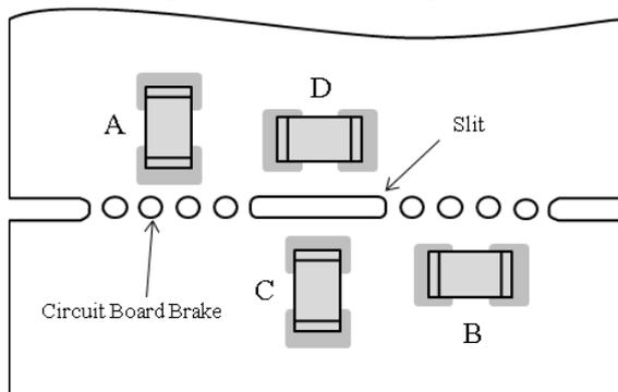
Stress strength according to the mounting position:
