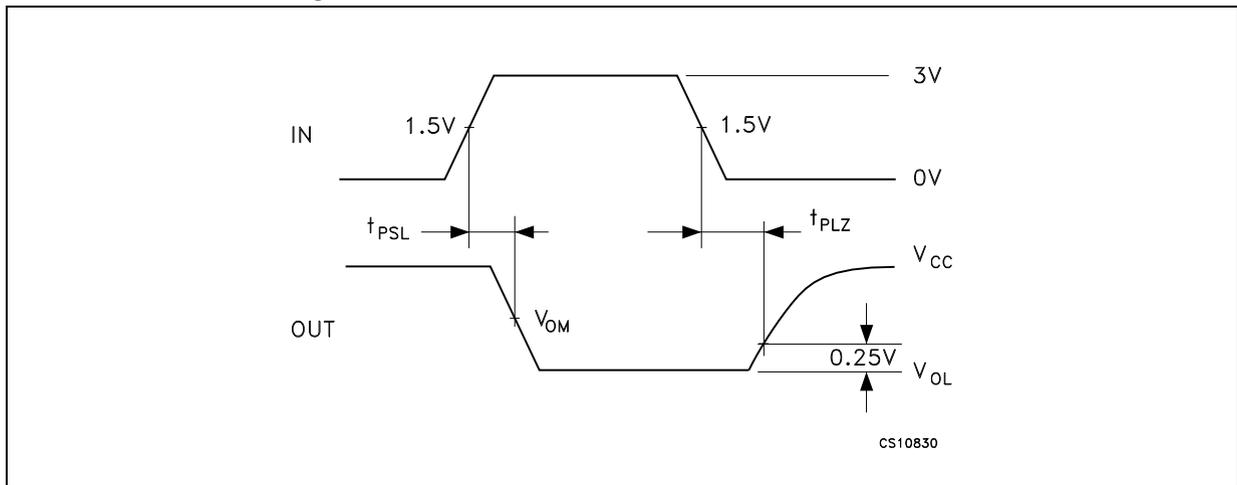
Figure 14. Receiver propagation delay time test circuit
