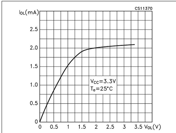
**Figure 22. Receiver output current vs output high voltage**
