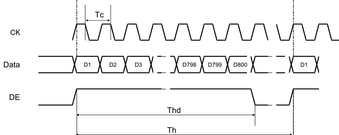
8-2. Input Data Signals and Display position on the screen
