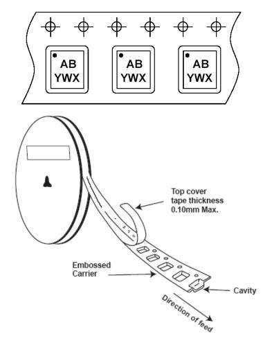
Notes: 8. The taping orientation of the other package type can be found on our website at <a href="http://www.diodes.com/datasheets/ap02007.pdf">http://www.diodes.com/datasheets/ap02007.pdf</a>.
