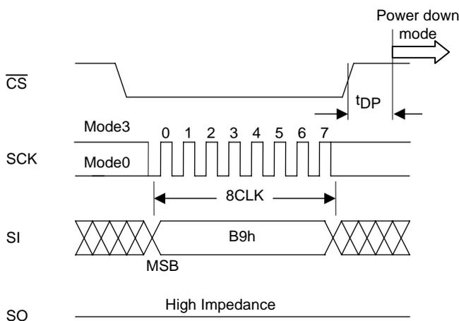
**Figure 11 Exiting from Power-down**
