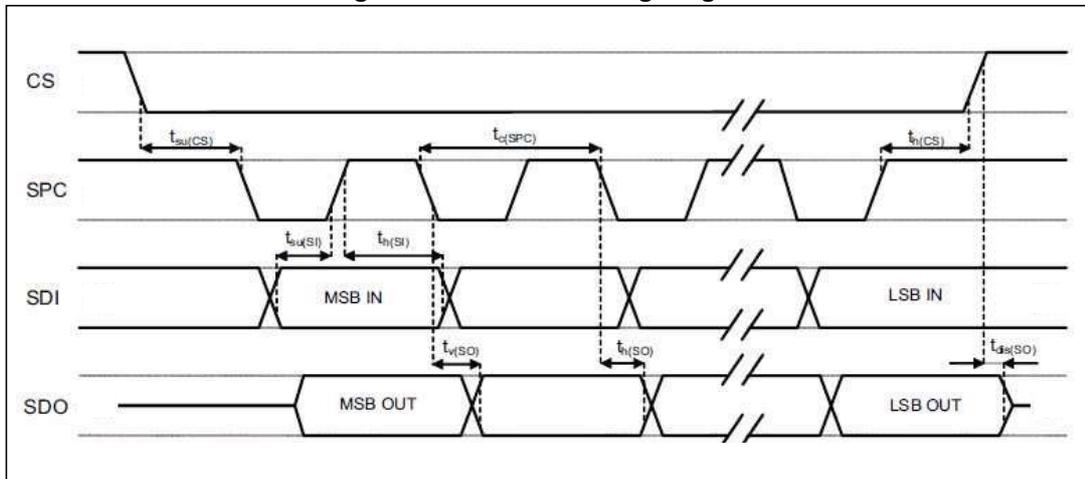
Note: Measurement points are done at 0.2·V<sub>DD\_IO</sub> and 0.8·V<sub>DD\_IO</sub>, for both ports.
