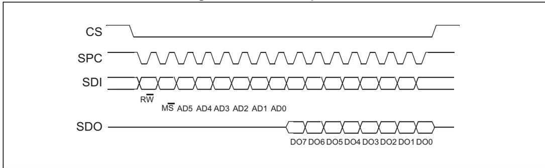
The SPI read command is performed with 16 clock pulses. The multiple byte read command is performed by adding blocks of 8 clock pulses to the previous one.
