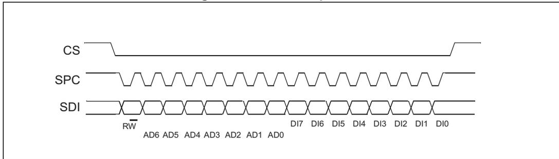
The SPI write command is performed with 16 clock pulses. The multiple byte write command is performed by adding blocks of 8 clock pulses to the previous one.
