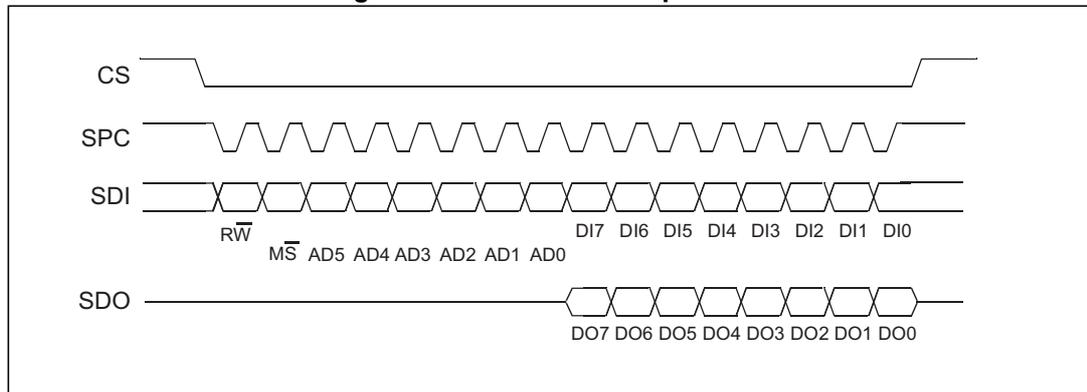
**CS** is the serial port enable and it is controlled by the SPI master. It goes low at the start of the transmission and returns to high at the end. **SPC** is the serial port clock and it is controlled by the SPI master. It is stopped high when **CS** is high (no transmission). **SDI** and **SDO** are respectively the serial port data input and output. Those lines are driven at the falling edge of **SPC** and should be captured at the rising edge of **SPC**.
