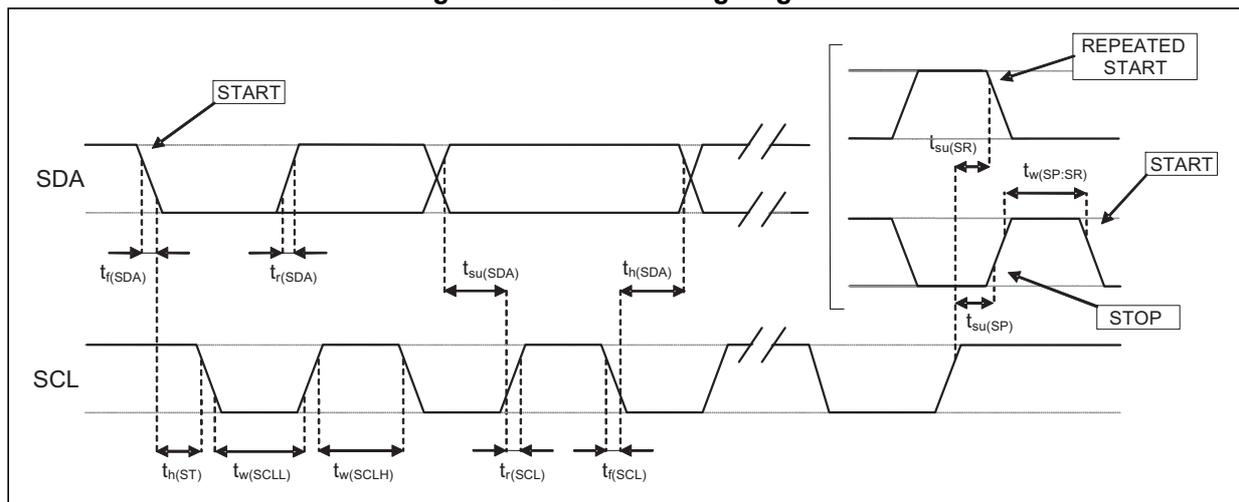
Note: Measurement points are done at 0.2·V<sub>DD\_IO</sub> and 0.8·V<sub>DD\_IO</sub>, for both ports.
