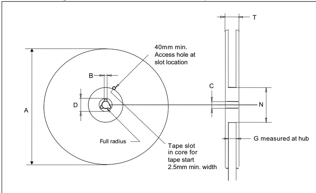
Table 25. Reel dimensions for carrier tape of HLGA-10L
