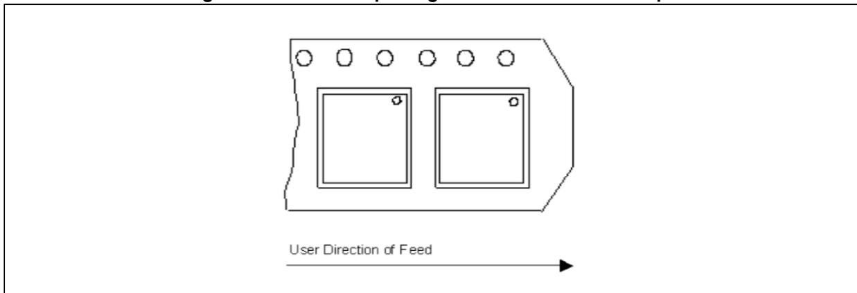
Figure 25. Reel information for carrier tape of HLGA-10L
