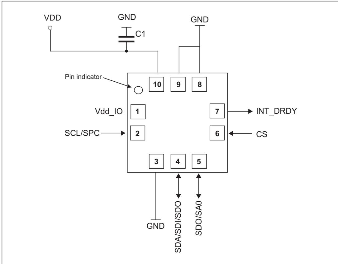
The device power supply must be provided through the VDD line; the power supply decoupling capacitor C1 (100 nF) must be placed as near as possible to the supply pads of the device. Depending on the application, an additional capacitor of 4.7  $\mu$ F could be placed on VDD line.
