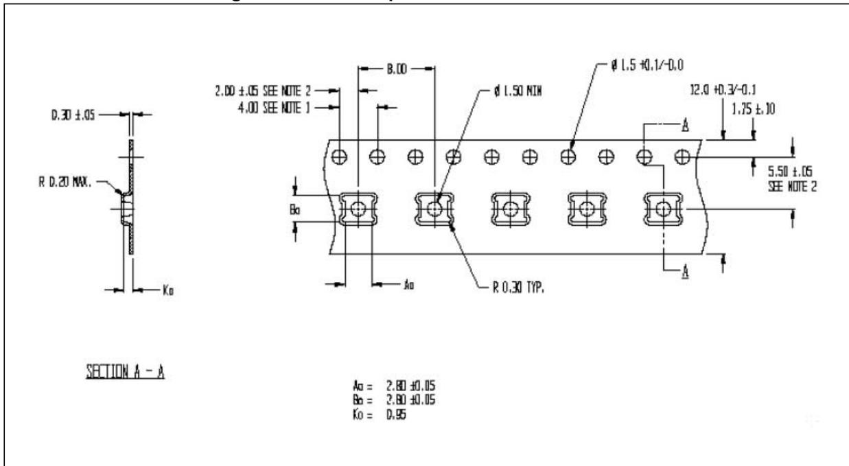
Figure 24. HLGA-10L package orientation in carrier tape
