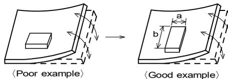
(2) Components location on PCB separation
