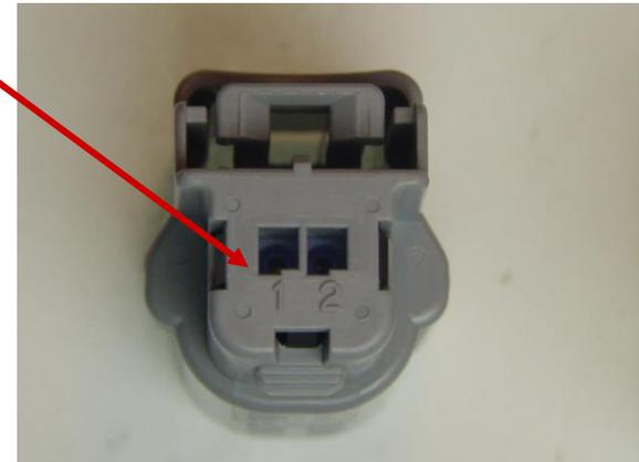
**Terminal Insertion Orientation to Grommet Seal Cover**
