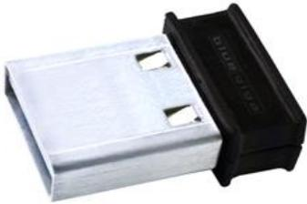
**Figure 1: BLED112 Bluetooth Low Energy USB dongle**
